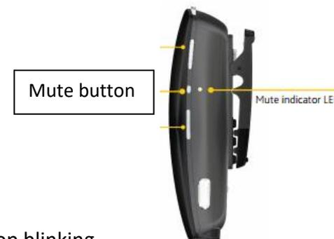
1. Teacher to turn off the MM2+ by pressing the ON/OFF button until the LED turns red, then release the button.
