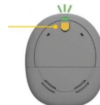
Alternatively, streaming can be turned off with the Remote Assistant by one quick press on the Telecoil button or by selecting OFF on the Stream screen.
