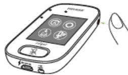
4. \*Hold the transmitter within 4 inches of EACH receiver and tap *Connect*.
